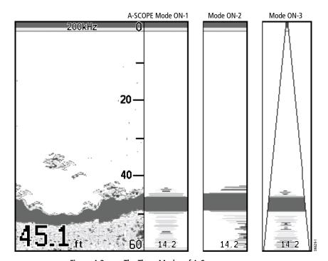
Figure 4-2: The Three Modes of A-Scope
